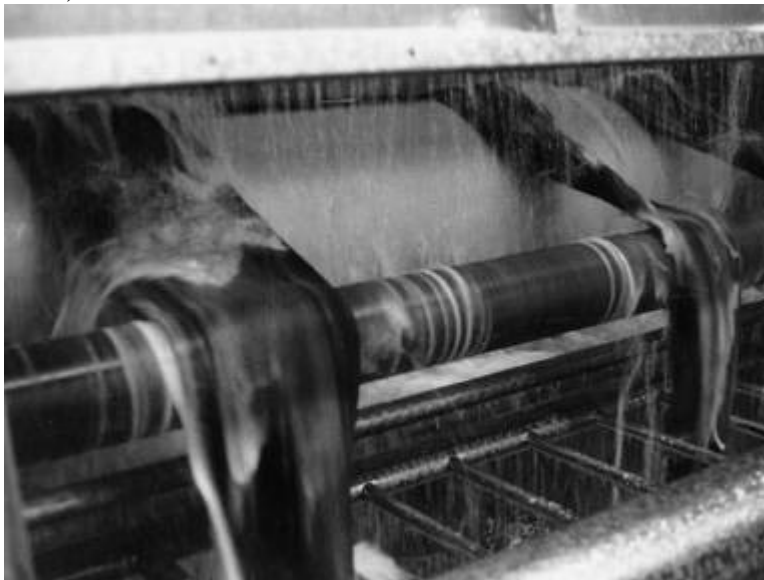
A rope scouring and milling machine used in fabric finishing.
